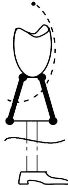
Fig. 5. Scheme of a four-axial mechanism for a prosthetic knee. The dotted line represents the path followed by the centre of rotation cr . The big dot represents the cr when the knee is extended. Placing this point more backward, results in a more stable stance phase
