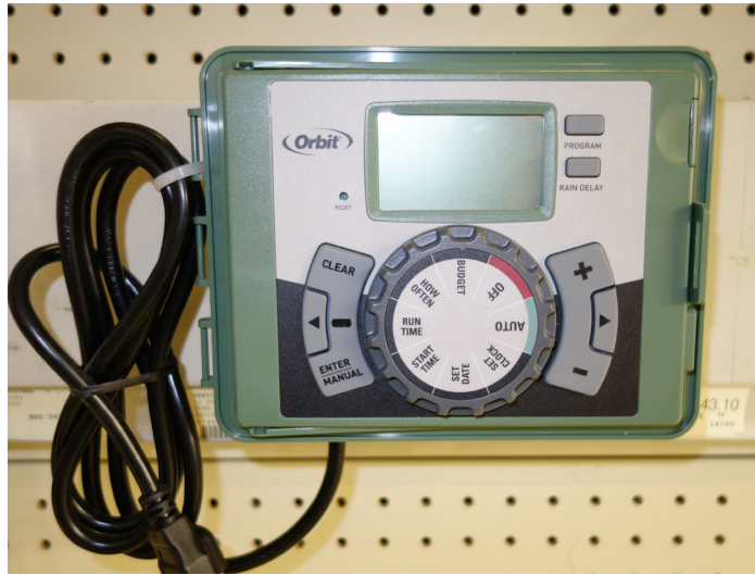
Figure 16. A programmable irrigation controller for multiple zones. More advanced units can become “smart” with the addition of soil moisture sensors and weather sensors.
