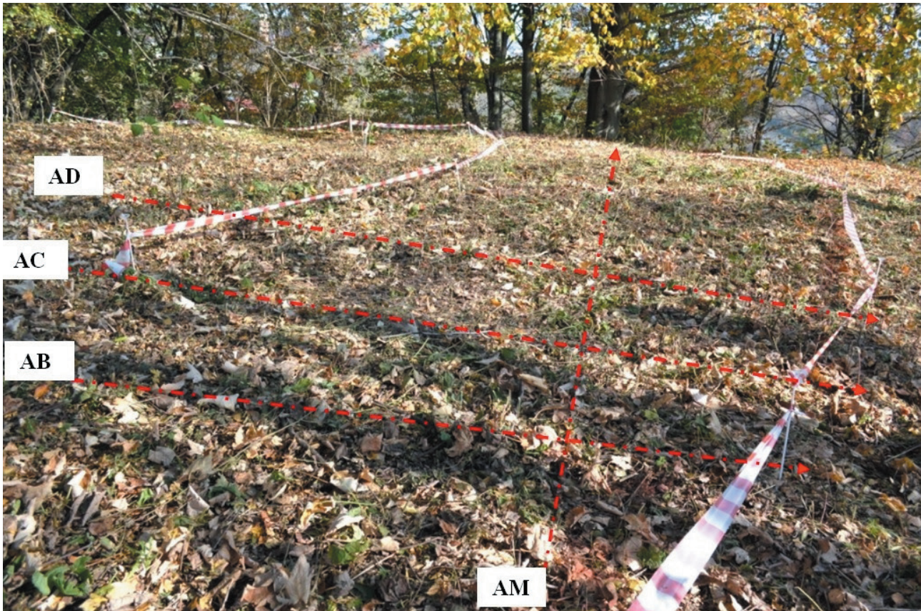
Fig. 9. The schematic distribution of GPR profiles on the investigated site 1a (prepared by B. Rajchel 2019)
