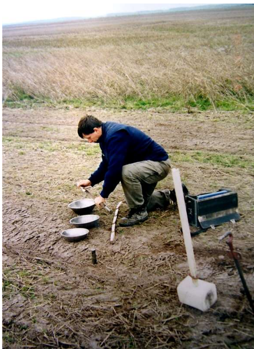
Figure 7: Transferring the different soil depths (0 - 30 cm, 30 - 60 cm 60-100 cm) in bowls for evaluation in the field (photo: LMBV 2006)
