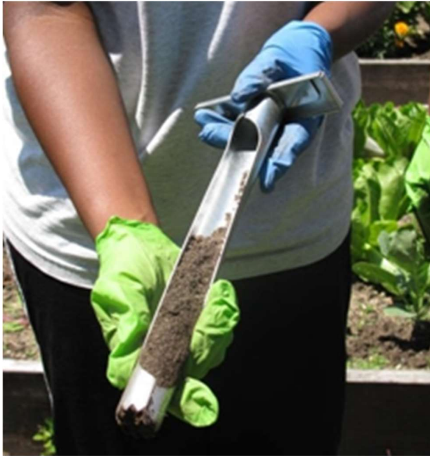
Figure 5: Typical soil-auger (photo: Robin Simmen, Cornell University)
