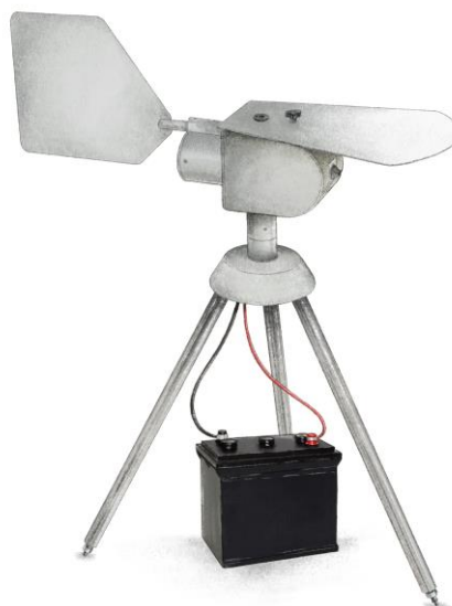
Figure 4.1. Hirst-type, 7-day recording volumetric spore sampler VPPS 2000 (Lanzoni) (Drawing by Quim Pallarès, 2020).
