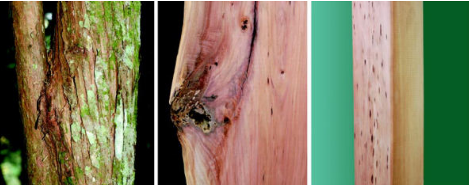
The pocket of rot in the sawn board (right) has resulted from a steep angle branch similar to that on the stem (left). Removal of these large upright branches and any double leaders as soon as they can be identified is likely to reduce defect in the wood.
