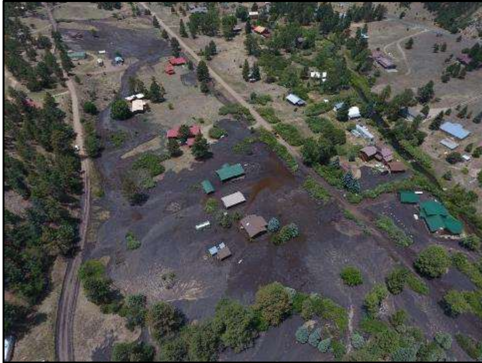
Figure 1.3. Debris flow generated from the Ute Park Fire that impacted Ute Park on July 13, 2018, following approximately 0.3 inch of rain directly on the burn scar upslope from Ute Park.
