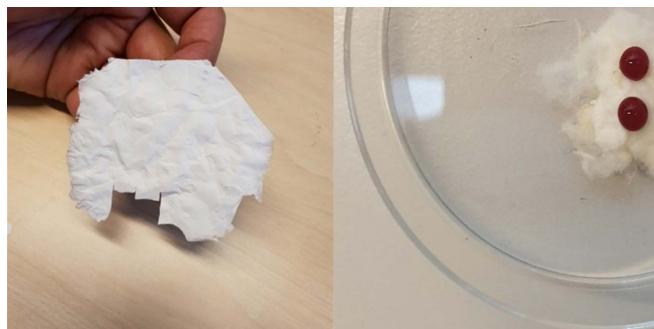
Fig. 3. Plant protein based textiles of various types and their absorption properties; a) paper-like gliadin fiber mat; b) wheat gluten textiles absorbing blood. Photos by Ramune Kuktaite
