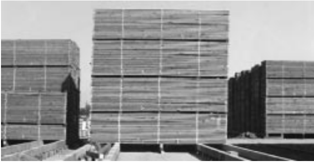
Figure 13–8. A sanitary, well-drained air-drying yard.
