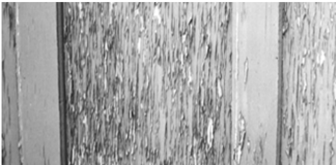
Figure 15-4. Early paint failure on plywood caused by penetration of moisture into surface face-checks.
