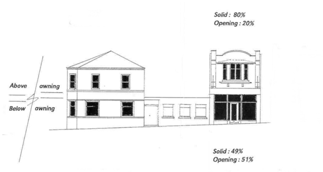
Figure HOB-S2.3 Building Form: Solid / Void Ratio, example of building with appropriate solid to void proportion.
