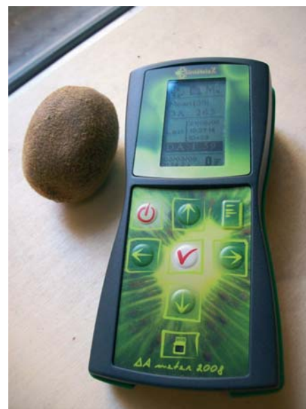
Kiwi-Meter, a non-destructive device for fruit quality assessment.
