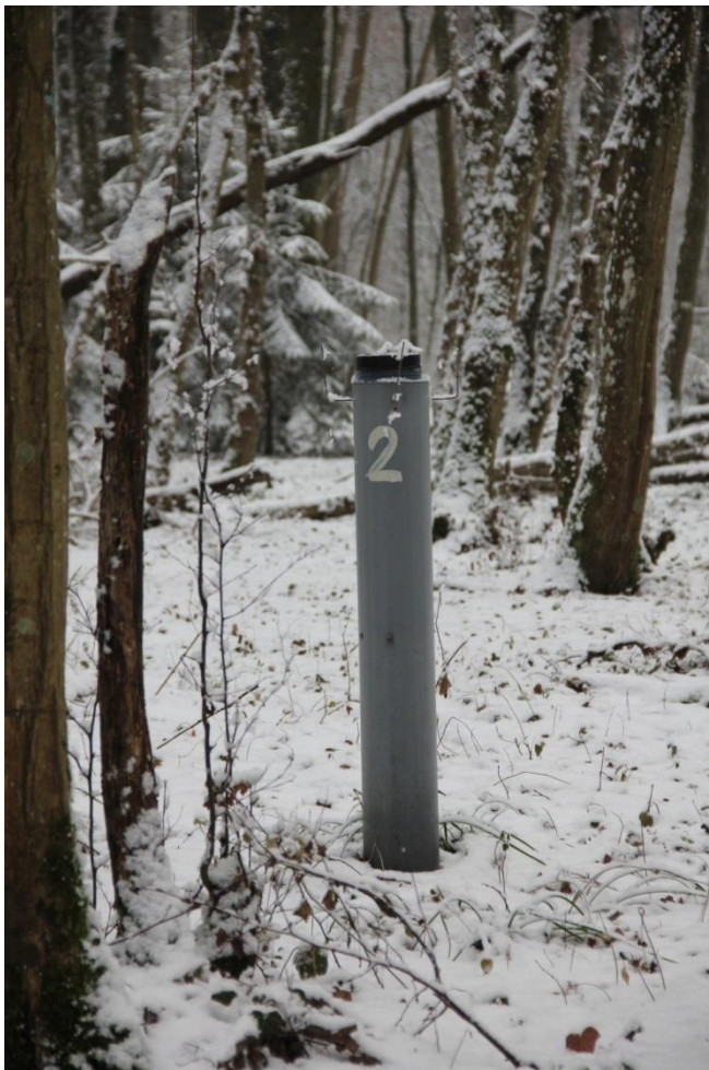
Figure 5-1: Throughfall deposition sampler on a Level II plot in Switzerland close to Geneva (Image: Peter Waldner, WSL)
