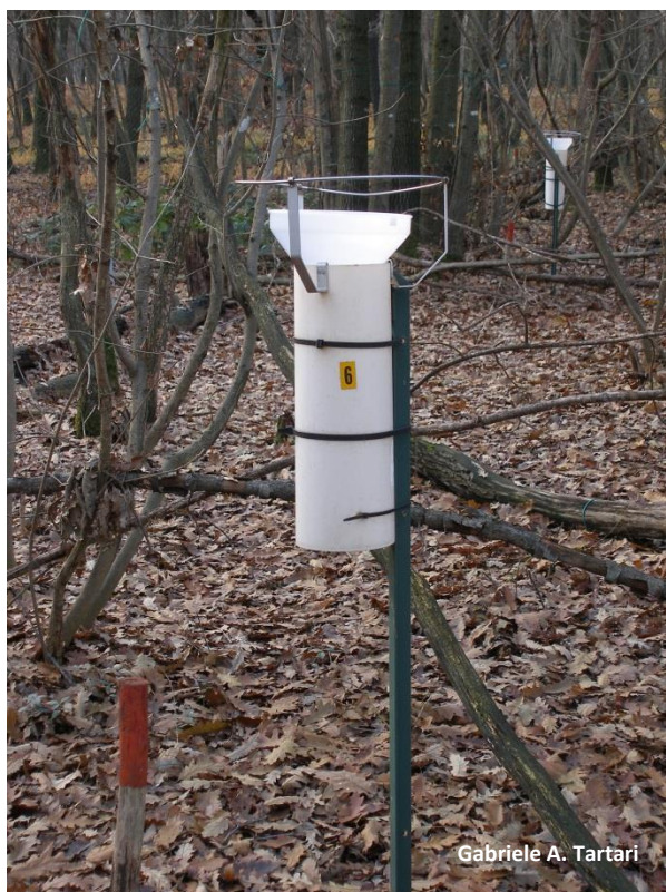
Figure 4-1. Deposition sampler located under forest canopy to collect throughfall in Italy.
