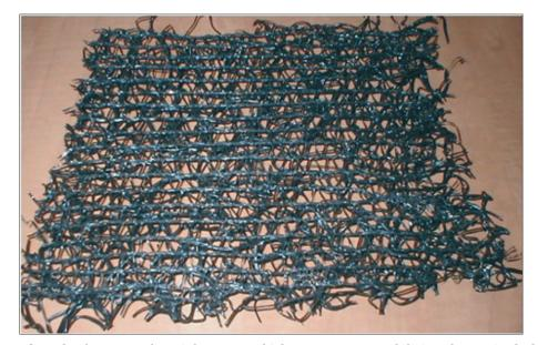
*Fig. 3: Sample of one type of spatial geonets, which can serve as a stabilizing element in the body of the slope (photo M. Šlezingr)*
