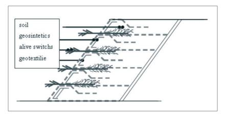
Fig. 4: Shoreline stabilization scheme (Úradníček, Šlezingr, 2007)
