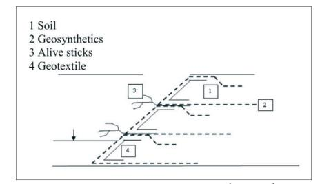
Fig. 5: Reinforced structure combined with vegetation - scheme (Úradníček, Šlezingr, 2007)
