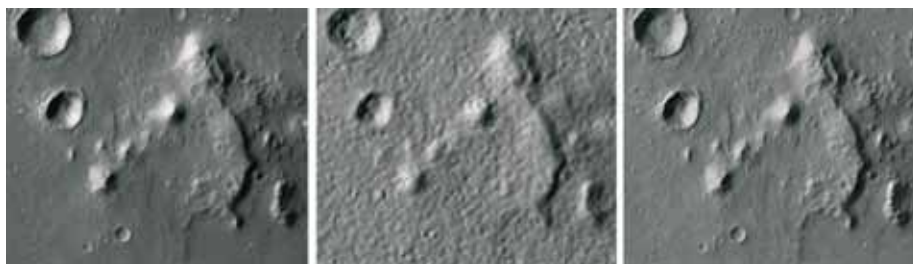
Fig. 9. A 495 \times 565 subsection from HRSC orbit 927 with 50 m ground pixel size (scene size 25 \times 28 km). (a) Photometrically corrected irradiance of the original orthoimage derived from the corresponding HRSC nadir image and a standard Level-4 DTM. (b) The modelled scene radiance of this obviously relatively crude DTM. (c) The modelled scene radiance of the SFS-refined DTM. The fact that (c) is almost indistinguishable from (a) demonstrates the potential of SFS.
