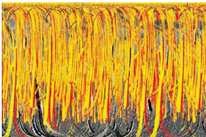
Fig. 1. PFS coverage of Mars up to 18 April 2005, after more than a year of operations. The vertical axis shows latitude, the horizontal axis shows longitude. The footprint of the LW channel is in red (if with solar illumination), while the SW footprint is in yellow. The grey footprints indicate no solar illumination.
