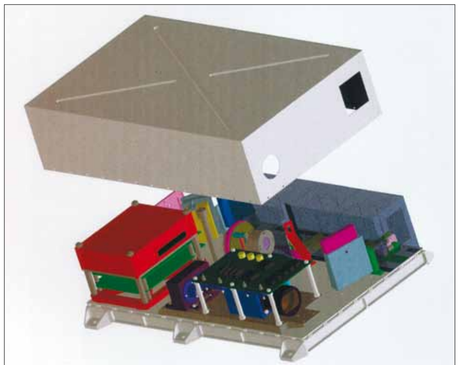
Fig. 1. Mechanical layout of the SUV and SIR channels. The IR AOTF spectrometer is at the front; the UV spectrometer is at the rear. The common optical axis points to the right (the +Z axis of the spacecraft).
