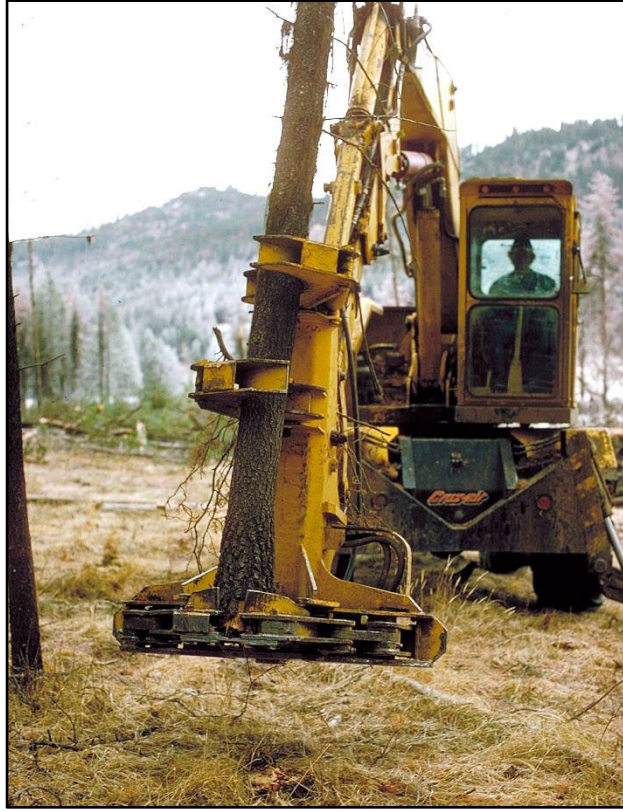
Figure 38 – Tree shear harvest system (clipper) harvesting a lodgepole pine, Umatilla NF. This type of shear was used to harvest much of the beetle-killed timber during the mid-1970s mountain pine beetle outbreak, and because it has a relatively short articulating arm, the shear had to get close to each tree to remove it; this resulted in compacted soils for a high proportion of the harvested sites (Geist et al. 2008). The Heppner RD completed more than 10,000 acres of soil compaction remediation treatments (e.g., sub-soiling) in the late 1980s and 1990s to ameliorate shear-caused soil compaction.
