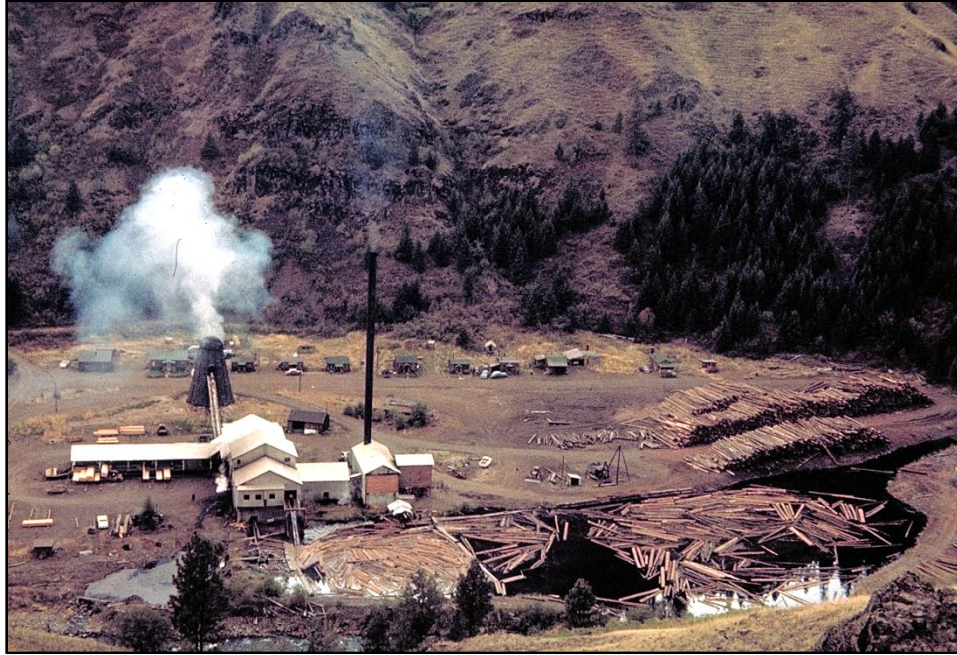
Figure 59 – Sawmill located at Troy, Oregon, showing associated log holding pond, log decks, and a teepee-style burner for disposing of sawdust and other milling waste. From the 1950s through the 1970s, almost every community in eastern Oregon had at least one wood-processing facility (Gedney 1963).
