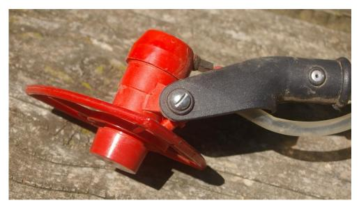
Figure 9.7 - Controlled droplet (spinning disc) nozzles could potentially be used to apply herbicide from on drones. They use low volumes and create large droplets, which would reduce non-target damage.
