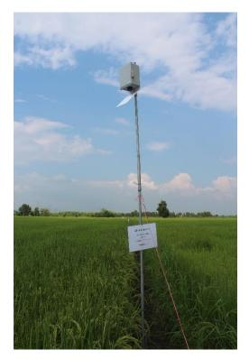
Figure 13.1 A bat acoustic monitoring station; a bat detector is kept in the box (Photo: Sara Bumrungsri)
