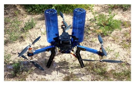
Figure 7.2 - 3D-Robotics' Y6 hexacopter adapted to carry two seed dispensers
