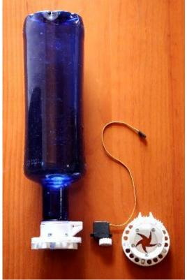
Figure 7.6 – Controlled by mobile phones with open-source software and constructed from open-source hardware, with biodegradable wooden frames, "flones" are inexpensive and easily repaired. Thus, they are ideal UAVs for citizenbased ecological actions.
