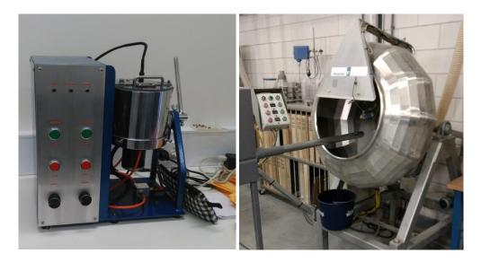
Figure 8.3 – Seed-coating equipment, lab-scale rotary coater on the left, rotating pan on the right.
