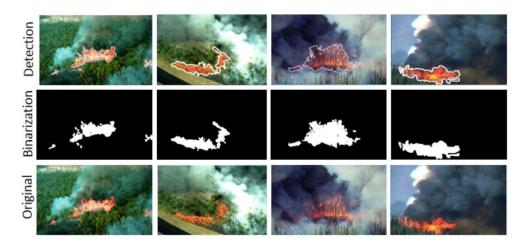
Figure 2.2 – Forest fire detections from UAVs (modified from Cruz et al., 2016)
