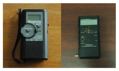
Figure 13.2 A heterodyne bat detector (left) and a time expansion bat detector (right) (Photo: Sara Bumrungsri)
