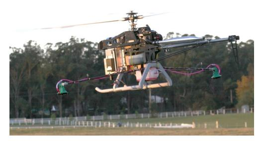
Figure 9.6 – An auto-piloted mini helicopter, used for weed control
