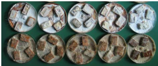
Photo 3. Samples of TMW after 16 weeks of impact of T. versicolor (up) and C. puteana (down); From left to right: Control; 100 °C; 140 °C; 170 °C; 200 °C;
