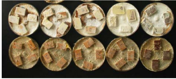
Photo 1. Samples of TMW after 8 weeks of impact of T. versicolor (up) and C. puteana (down). From left to right: Control; 100 °C; 140 °C; 170 °C; 200 °C;
