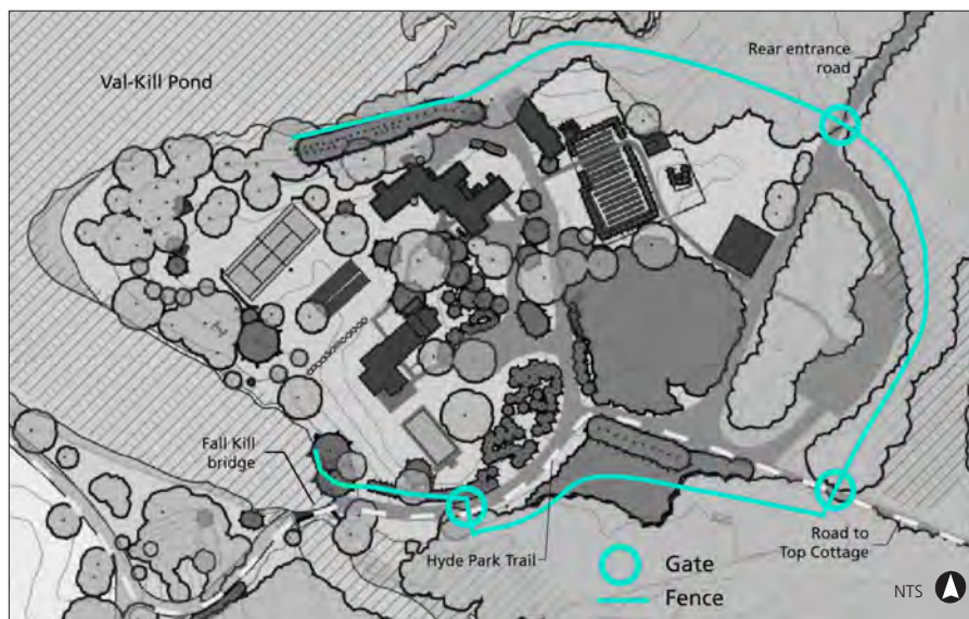
Figure 2.6. Potential location of a site-wide deer fence around the historic core to protect shrubs and herbaceous plantings that are susceptible to deer browsing year-round. (SUNY ESF)
