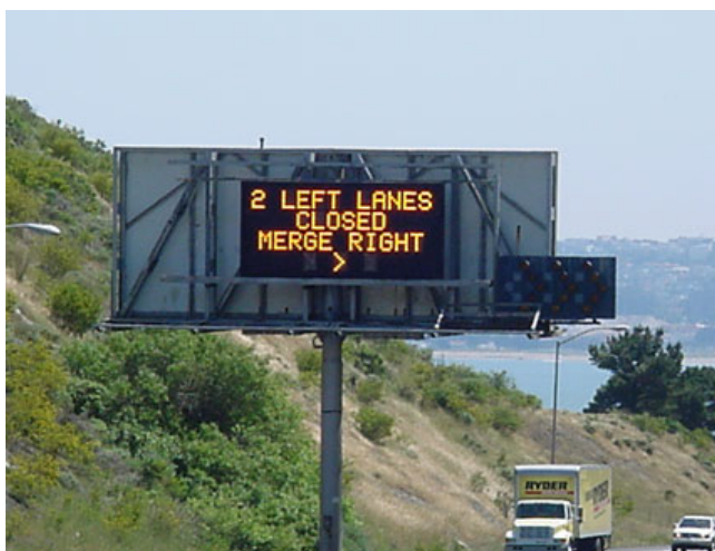
Example of a variable message board ( http://www.oksolar.com/visual_signals/heavy-traffic-signs.htm )
