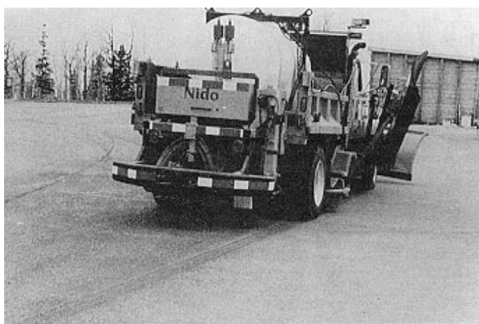
Liquid spread unit set in dump truck body (FHWA Effective Anti-Icing Program 2004)
