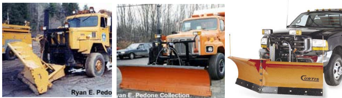
One-Way Snowplow (www.hankstruckpictures.com), Reversible Snow Plow (www.hankstruckpictures.com), and a Four-Way Snowplow (www.curtisplow.com)
