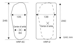
Fig. 4 Size of left soles and the central position of the ankles of HRP-4C and HRP-2
