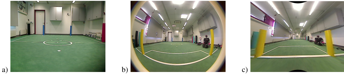
Fig. 5. Wide-angle lens: a) A raw camera image of a RoboCup soccer field without the wide-angle lens. b) An image from the same perspective using the wide-angle lens shows the increased field of view and the introduced barrel distortion. c) Undistorted camera image computed using Eq. 1.
