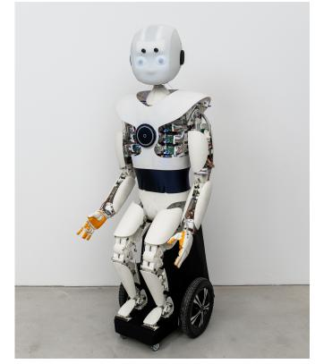
Fig. 1. Tendon-driven humanoid robotic avatar Robody
