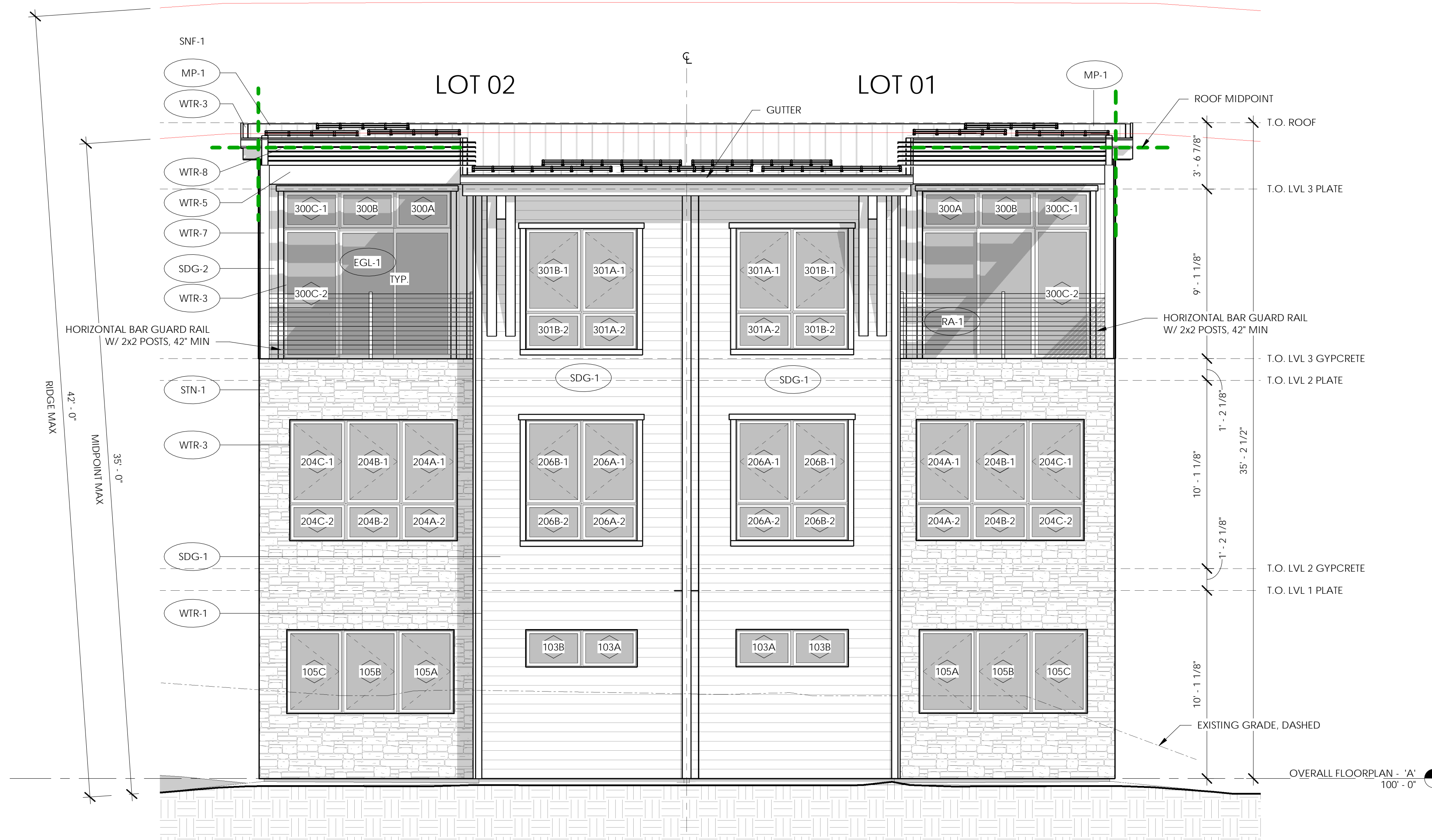
1 OVERALL BUILDING ELEVATION - BUILDING 'A' SOUTHEAST A3.04 SCALE: 1/4" = 1'-0" BACK REF: A3.01
