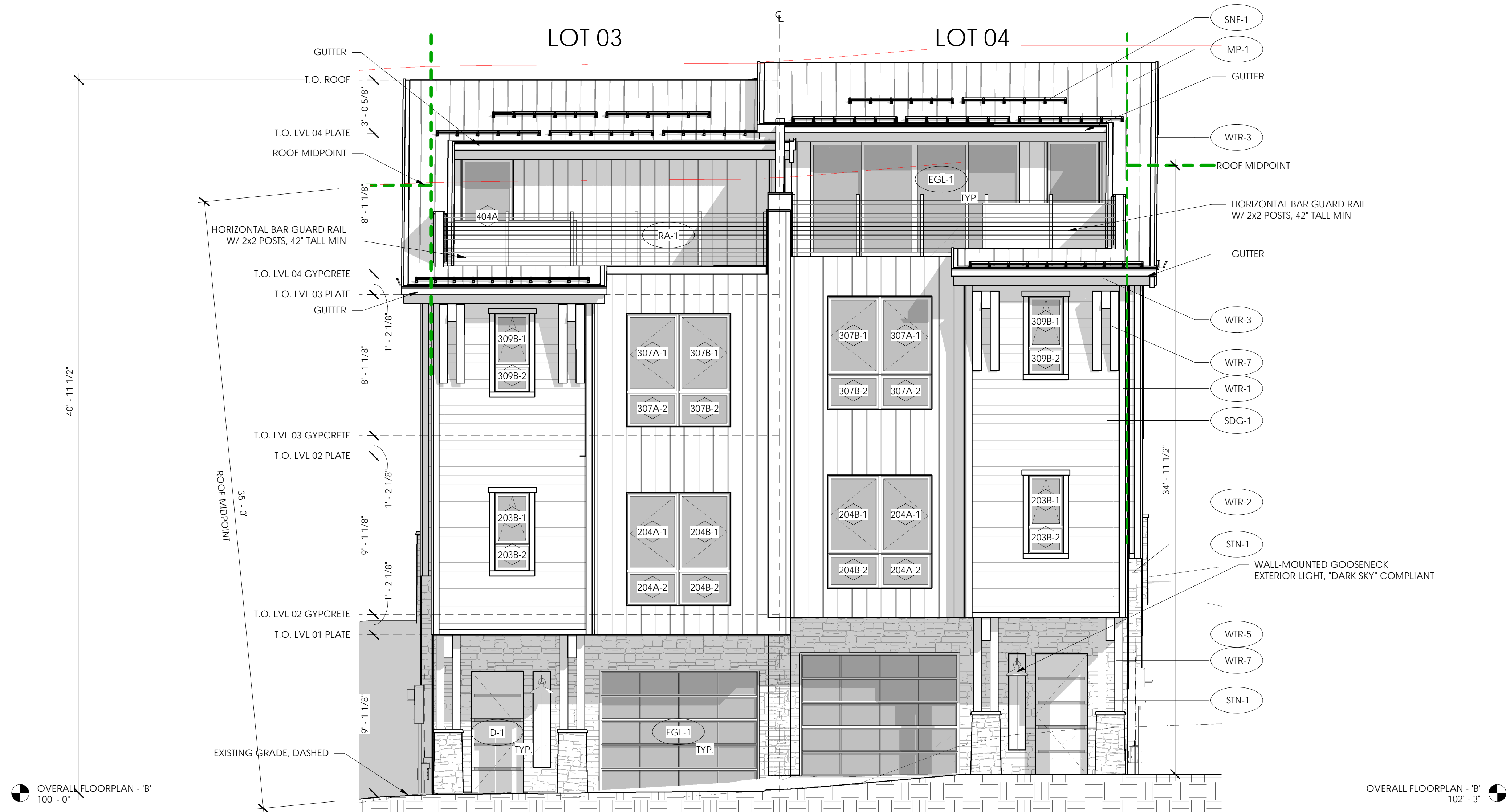
1 OVERALL BUILDING ELEVATION - BUILDING 'B' EAST A3.11 SCALE: 1/4" = 1'-0" BACK REF: A3.01
