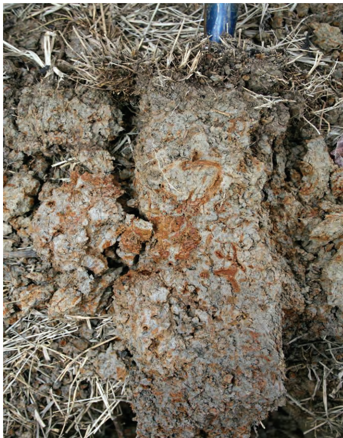
Figure 24. This soil has a depleted matrix with redox concentrations in a low-chroma matrix.
