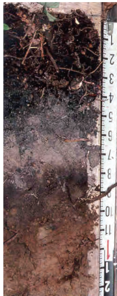
Figure 21. Example of the Thin Dark Surface indicator. A spodic horizon is present starting at 8 in. (20 cm). Scale is in inches.
