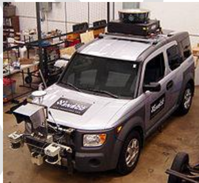
RADAR, GPS, LIDAR, ... are all combined to provide proper navigation and obstacle avoidance
