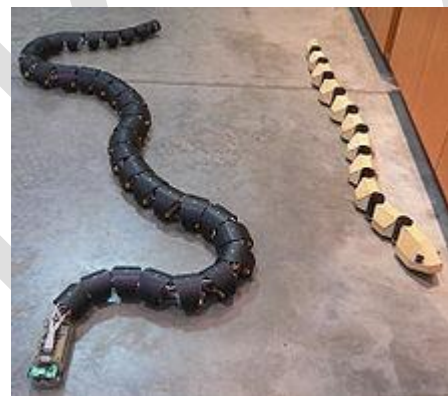
Two robot snakes. Left one has 64 motors (with 2 degrees of freedom per segment), the right one 10.
