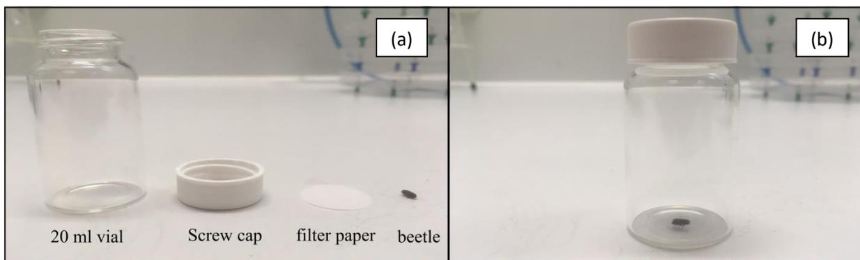
**Figure 5:** Experimental setup for fumigation toxicity assay. (a) Materials used in the experiment, (b) the complete setup of the experiment where a single beetle is placed at the bottom of the glass vials and the filter paper containing test chemical was secured on the top under the lid.
