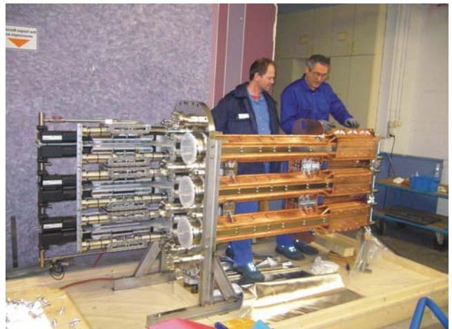
Figure 32: ECRH front steering antenna module during final assembly at the central workshop of FZK. The three beamlines are clearly seen, each of them is equipped with independent bi-axially movable front mirrors.
