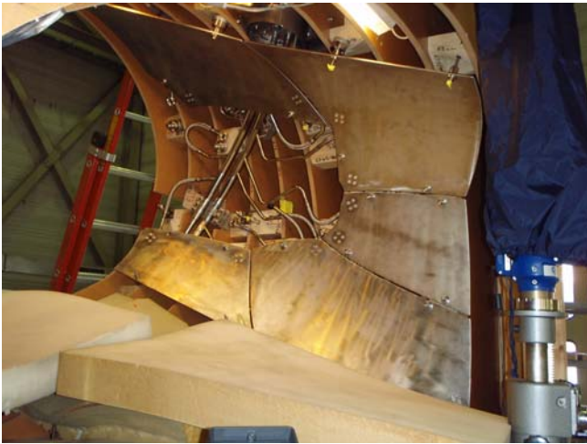
Figure 8: Test assembly of pipe work and panels in the wooden mock up
