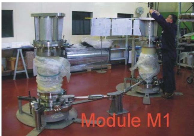
Figure 3: Acceptance test of Cryolegs M1 1
