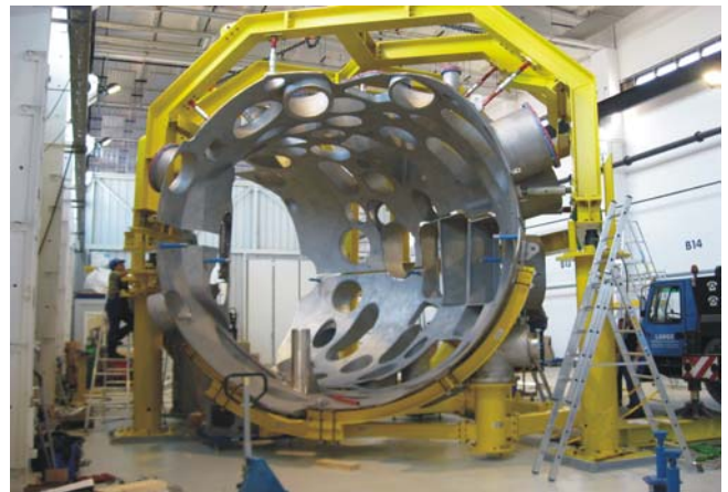
Figure 20: Preparation outer vessel shells
