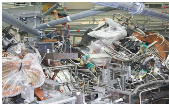
Figure 22: Assembly, welding and leak test of pre-band He-pipes
