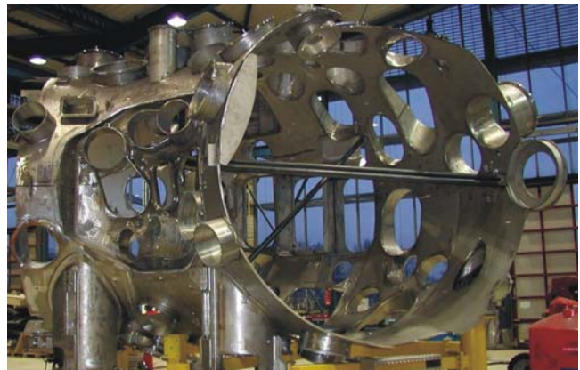
Figure 5: Pre-assembled lower and upper shells of module 5
