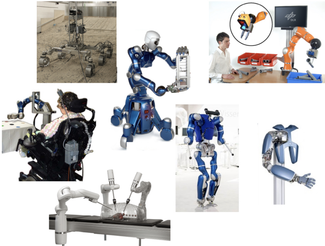
Figure 2.12: Robotic domains in which the aRD and aRDx frameworks are used. Clockwise, starting in the upper left: ExoMars Rover, Agile Justin, human robot cooperation (HRC), DLR antagonistic humanoid HASy, DLR bipedal humanoid Toro, MiroSurge, Brain-controlled assistant. (Pictures are taken from the corresponding publications as referenced in Sec. 2.5.3.)
