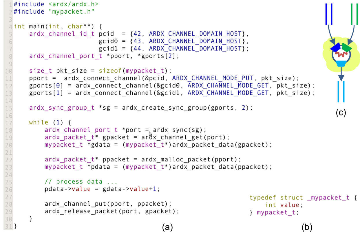
Figure 2.10: The C-source-code in (a) shows a fully functional aRDx-client-program that works on structs of the type mypacket_t given in (b). As illustrated in the abstract view (c), the example program consists of a single process with a single thread. It can read data from two get-ports, both inside a sync-group, connected to two different channels. A single put-port allows to send data to a third channel. The program is composed of the the specification of the used channels (L5–7), followed by the connection of the three ports to these channels resulting in two get- and one put-port (L11–13). Both get-ports are combined in one sync-group (L15). The main processing loop first waits via sync on new data on one of both get-ports, then retrieves a handle to the packet and a pointer to the data area from the returned port (L18–20). After allocating a packet-handle for the put-port, together with a pointer to its data area (L22, 23), both data pointers are accessible. This allows to generate the outgoing data in-place (L26). Afterwards, the outgoing packet is sent and the incoming packet is released.
