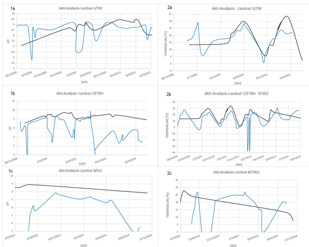
Fig. 3 pH (1) and Water Temperature (2) variations over the two sampling stations (Vasiloudi, Akti Analipsis) in pairs of time-series (2009–2014) from in situ data and data derived from suitable radiometric calibration of the thermal bands of the Landsat satellites.
