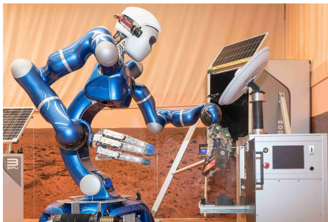
Fig. 1. DLR’s Rollin’ Justin replacing a defective component as commanded by the ISS crew during the METERON SUPVIS Justin experiment.
