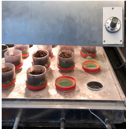
Figure 4.10.6 Automated heat and light extractor, with a temperature controlled top (heating) and bottom (cooling) chamber. Soil cores are placed on top of a mesh, and a collection beaker with preservative is placed below, cooled by the bottom chamber. Photo: Heidi S. Konestabo.
