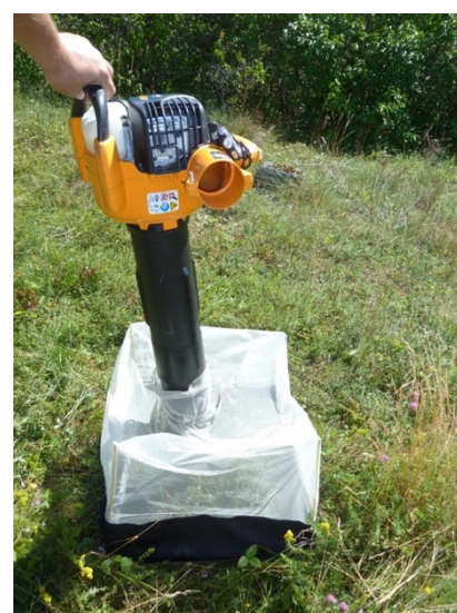
Figure 4.11.1 Vacuum or suction sampling in a closed area. Photo: Anders Endrestøl, NINA.
