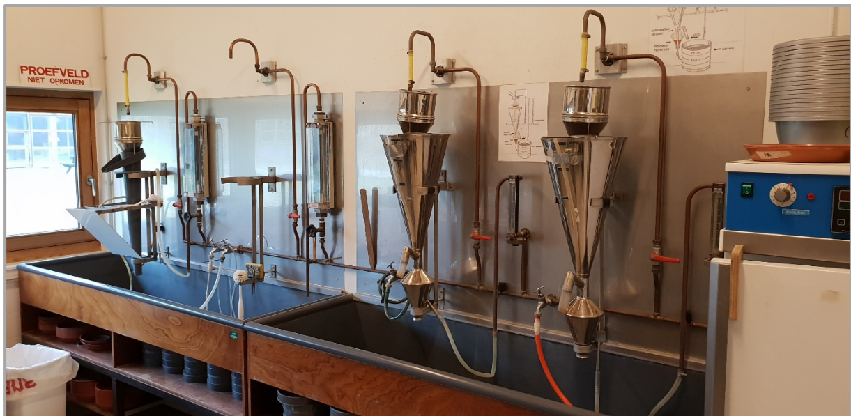
Figure 4.10.3 Oostenbrink elutriators at the Netherlands Institute of Ecology (NIOO-KNAW in Wageningen, the Netherlands). Photo: Freddy ten Hooven.
