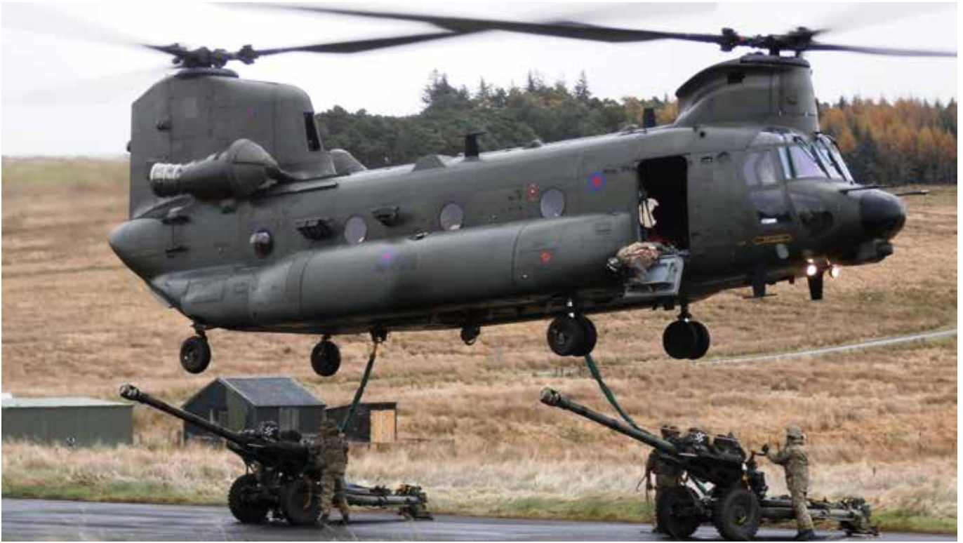
A chinook lifting two L118 light guns (a 105mm towed howitzer) on Otterburn Training Area © Crown
