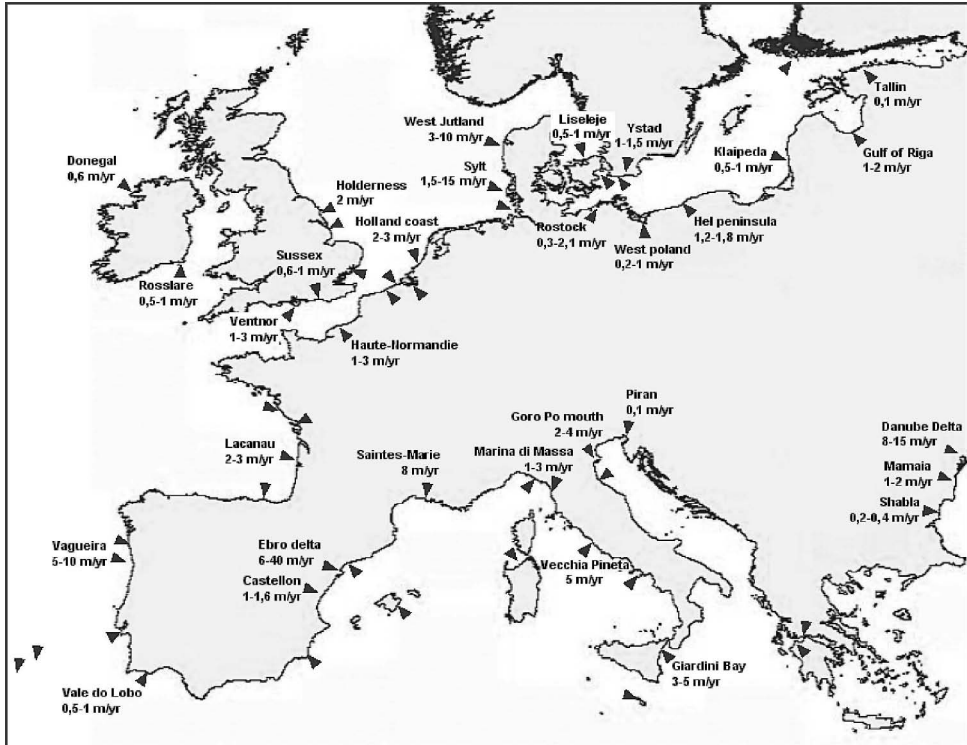
Fig. 1. Location of the 60 case studies reviewed during EUROSION study (with average erosion rate per year for selected cases).
