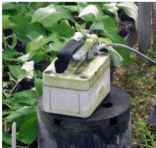
The Evaposensor helps detect and control the evaporative water demand on cuttings in a reliable and reproducible way
