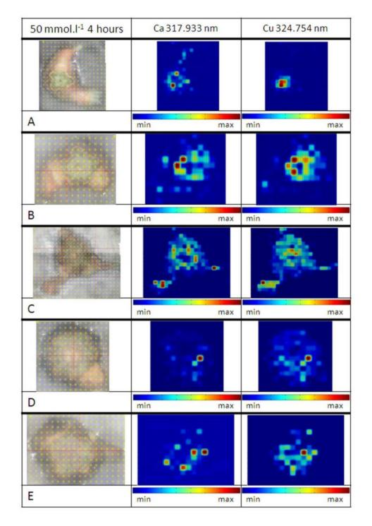
**Figure 3.** Series of the LIBS intensity maps showing the distribution of Ca (in the middle) and Cu (on the right side) on slices of stem of *Picea abies* (L.) Karsten. Other experimental conditions see in Experimental Section.
