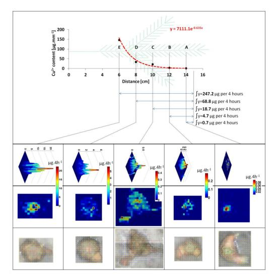
**Figure 8.** An application of integrals of area under the exponential curve made from ICP-MS data for specific distance intervals to LIBS intensity maps. 4 hours of cultivation in 50 mmol.l<sup>-1</sup> CuCl<sub>2</sub>. Other experimental conditions see in Experimental Section.
