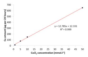
**Figure 9.** The relationship between CuCl<sub>2</sub> concentration of solution for treatment and total copper ions amount passed through E position after 24 hours. Other experimental conditions see in Experimental Section.
