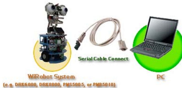
Figure IV.3 WiRobot System Setup without Wireless Connection
