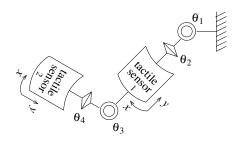
Fig. 3. Layout of joints and sensors
