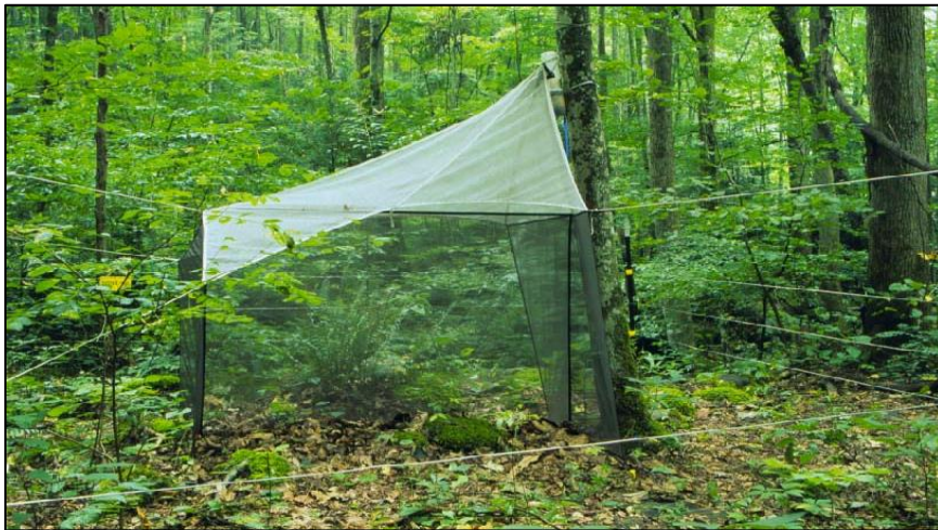
Figure 4.5.14.3. Malaise trap for flying arthropods. The insects self-collect in the collection bottle at the summit and are retrieved at set times, allowing for a quantified sample vs. effort catch. Source: NPS Photo 2014.
