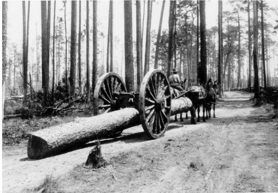
FIGURE 13. A “carry-log” drawn by mules. Economical range of this kind of transport was less than 4 miles (Croker 1987). Photo courtesy of U.S. National Archives.
