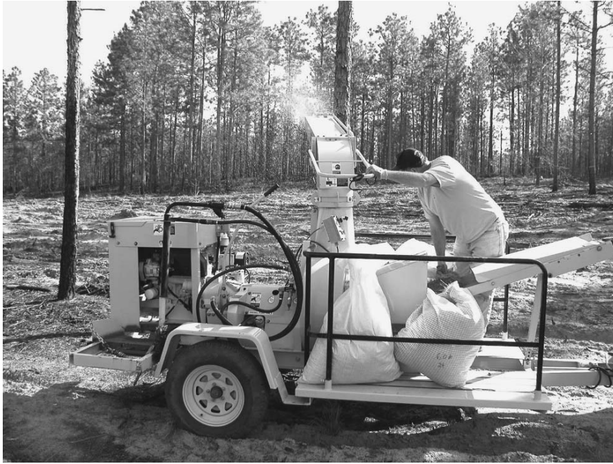
FIGURE 6. Standard hay blower distributing wiregrass seed at Fort Gordon, GA. This equipment is effective and widely available.
