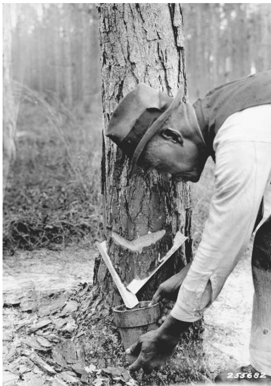
FIGURE 3. The Herty cup and gutter system for resin collection, circa 1906. Courtesy of USDA Forest Service. Image scanned from A Pictorial Album of the Naval Stores Industry (1937), University of Florida library.
