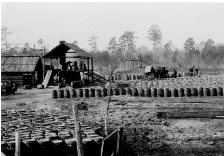
FIGURE 9. Introduction of the copper still into the woods in 1834 permitted reduction of crude gum to spirits of turpentine, saving shipping costs and making the process immensely more PROFITABLE. Photo courtesy of U.S. National Archives.
