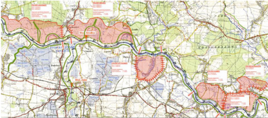
Fig. 7 The proposal of location of five flood polders in the valley of the River Vistula upstreams of Cracow for the reduction of flood peaks greater than 100-year flood: Self Source (Politechnika Krakowska)
