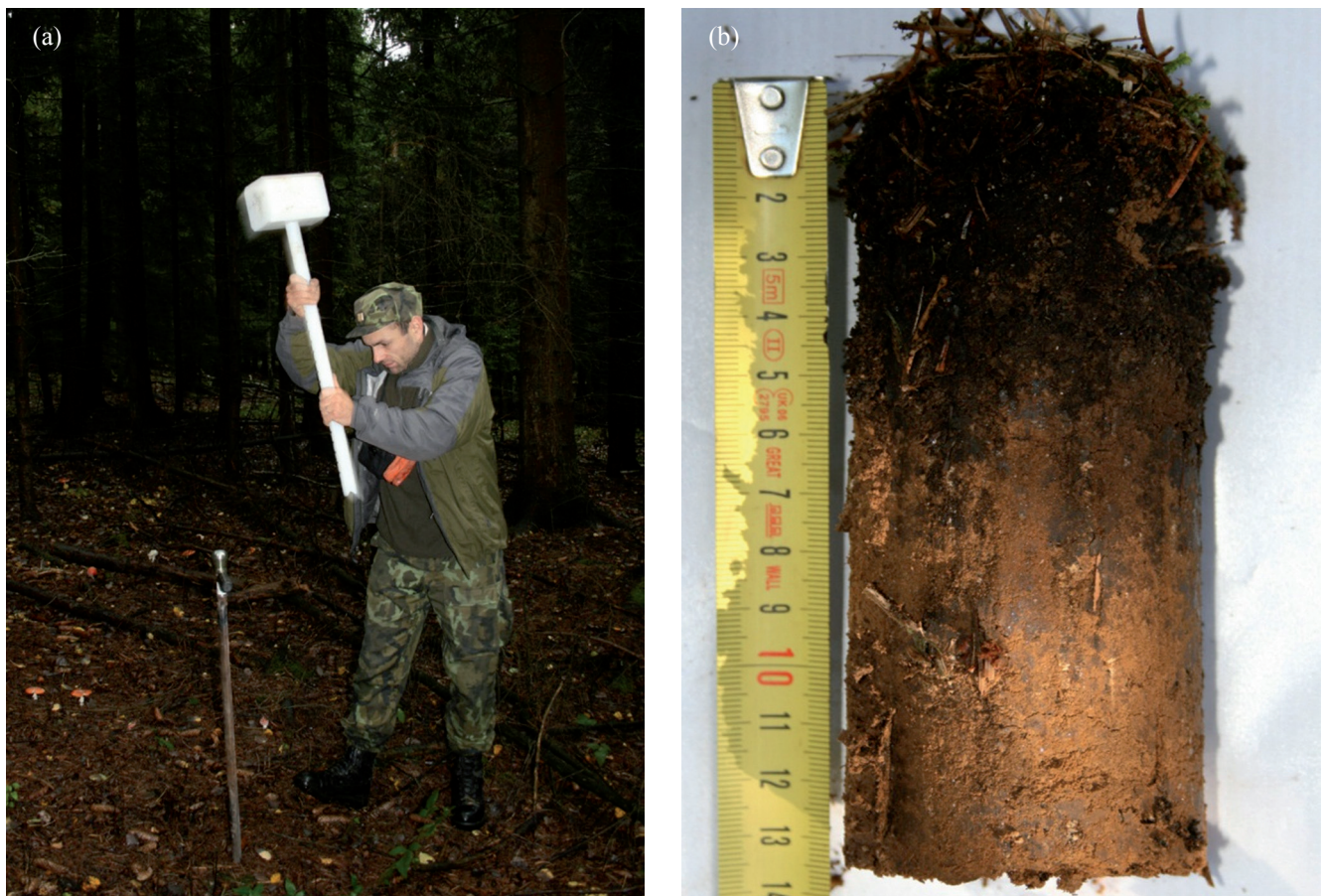
Figure 4. (a) The collection of soil samples by the soil probe (diameter 5 cm) at the deserted medieval village of Roudnička and an example of the soil sample collected from the deserted village of Spindelbach. The content of \delta^{15}\text{N} was only measured in the Ah horizon.
