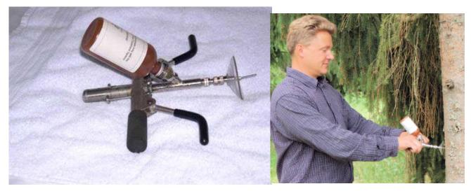
Figure 2. The Wedgle<sup>™</sup> Direct-Inject<sup>™</sup> tree injection unit from ArborSystems (Omaha, USA) tested in 504 Ålbrunna.
