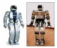
Figure 7: HUBO or KHR-3 (left) and its predecessor KHR-2 (right). Compared to the KHR-2, the HUBO is more streamlined and has smoother, more natural walking, has fingers instead of claws, voice recognition, and faster response times.
