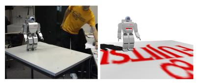
Figure 33: HOAP-2 and its Webots model performing a walk
