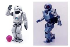
Figure 4: Sony Corporation originally developed a small biped walking robot "SDR" (3X and 4Xprototype). The right picture shows the SDR-3x. They are the previous series before the release of the QRIO (left)
