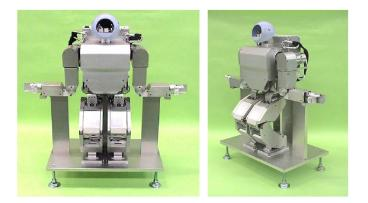
Figure 17: HOAP-2 initialization consists in putting the robot in a very precise position on a jig. The purpose of this manipulation is to put the robot on a known position (start position), and to pre-set the encoders counters of the joints in that posture. By knowing its start position, the robot can then calculate its current position.
